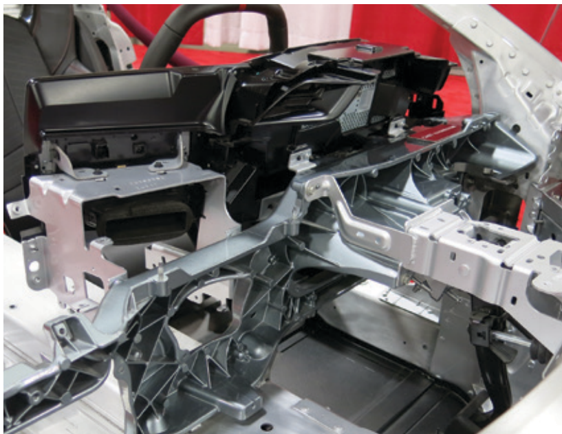
Details of C8’s magnesium crosscar beam and instrument module. Note deep-section center-tunnel structure.
