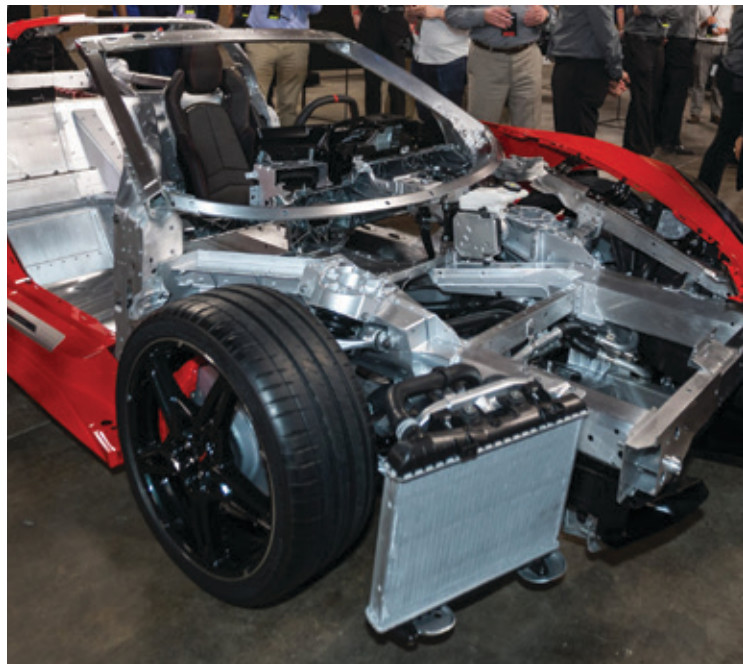
More 'Bedford' castings in C8's AL-intensive front structure. Note rear bulkhead and A-pillar construction, IP casting and coolant radiator location.
